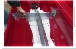
If the wipers are not lined up over the sponges or they need rotational adjustment on the shaft then loosen the 3mm grub screws and align. Place in the supplied baffle retaining baffle plates and tighten .
