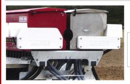
Test system and finally fit the supplied fibreglass cover if needed. Earlier drills without the fibreglass chain guards will need extra holes drilled in the cover to suit the existing mounting bolts.
